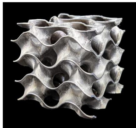
OrelTech silver layer on 3D printed PLA
