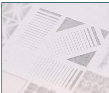
OrelTech Palladium ultra-thin Pd seed layer printed on PET
