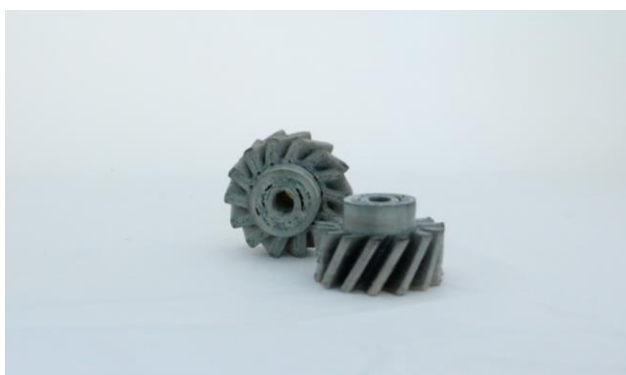
OrelTech silver electrode on 3D printed ABS
